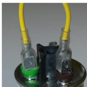
10.0 mfd - To configure the capacitor for 10.0 mfd a contractor would connect the one motor wire to the common and the other to the brown 7.5 mfd terminal. Then one jumper wire would be utilized to connect the brown 7.5 mfd terminal to the green 2.5 mfd terminal for a total 10.0 mfd.
