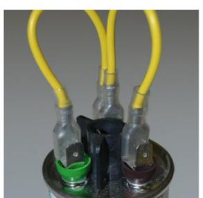
15.0 mfd - For applications requiring 15.0 mfd the two motor wires are connected one to the common and the other to the brown 7.5 mfd terminal. One jumper wire would then be utilized to connect the green 2.5 mfd terminal and the white 5.0 mfd terminal. The second jumper wire would then be used to connect the white 5.0 mfd terminal to the brown 7.5 mfd terminal for a combined 15.0 mfd.
