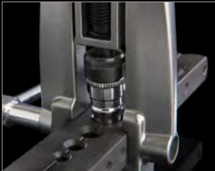
Push down the yoke and with fewer rotations, you get a precise flare or swage.
