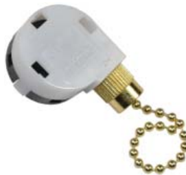
pull chain switch, 3 speed off-on-on-on, 6A/125VAC
