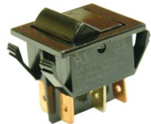
DPDT on-off-on rocker switch 16A 125/250 VAC / 10A 28VDC 6 terminals, ref. # 260411E approximate base size: 7/8 x 7/8"
