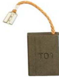
graphite brush, .221 x .647" 3/16" quick connect
