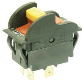
DPST, on-off safety switch removable lock, 4 terminals 20A @ 125-277VAC 1hp rating fits rectangular hole .80 x 1-7/16"
