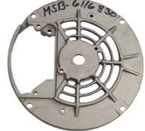
6.5" open non-drive endbell brg size : 6203 commonly seen on condensor fan motors
