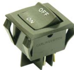
DPST on-off rocker switch 16A 125/250 VAC / 10A 28VDC 4 terminals, ref. # 260011E approximate base size : 7/8 x 7/8"
