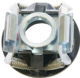
1725 rpm rotating mechanism / stationary switch kit mounting holes on switch : 3" c.-c. plastic spool o.d. 2-7/8" mechanism shaft size .950"
